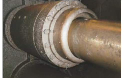
Spindle special seal for harsh environments.
