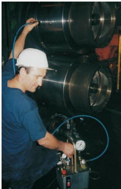
Pumping oil into a spindle with Safeset®
