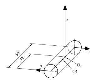
Special case of a), namely resultant unbalance vector located at the centre of unbalance CU. The associated couple unbalance is a minimum and lays in a plane orthogonal to the resultant unbalance vector
