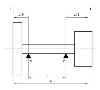
NOTE Tolerance (bearing) planes are A and B; correction planes are I and II.
