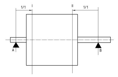
NOTE Tolerance (bearing) planes are A and B; correction planes are I and II.
