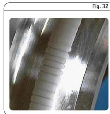
Washboarding caused by current leakage erosion
